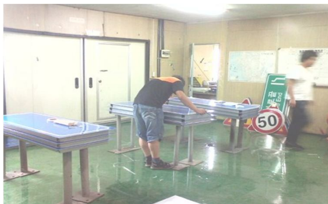
③ Adhere retroreflective sheets after the inspection of the painting.
