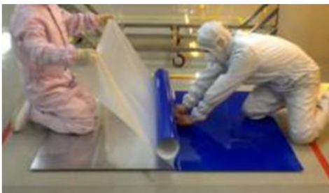
<Adhere the large retroreflective sheet.>
